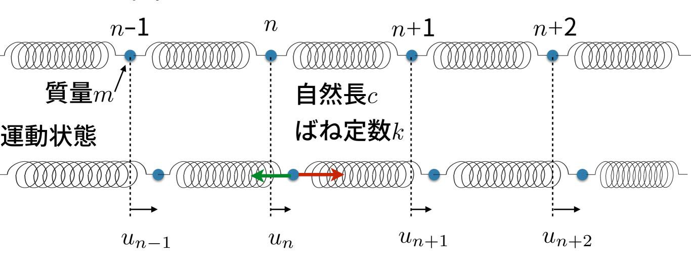
ばねののび:  $u_n - u_{n-1}$   $u_{n+1} - u_n$  質点nに働く力:  $-k(u_n - u_{n-1}) + k(u_{n+1} - u_n)$  (両端以外)
